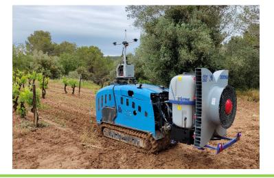
Autonomous robot for the treatment of rows of vines (also located in places with high slopes).
