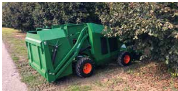
CORYL ROBOT: for the automated harvesting of hazelnuts.
